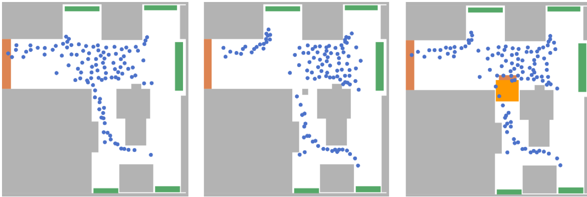
Figure 30: Cathedral area of Edinburgh, comparison of (left) no side street obstruction (control) (middle) obstruction on the side street and (right) attraction on the side street.
