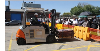
Fuel Cell powered forklift and refueling infrastructure deployment at Impala Platinum Refineries, Springs
