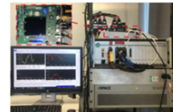
dSPACE and LabVIEW rapid prototyping hardware
