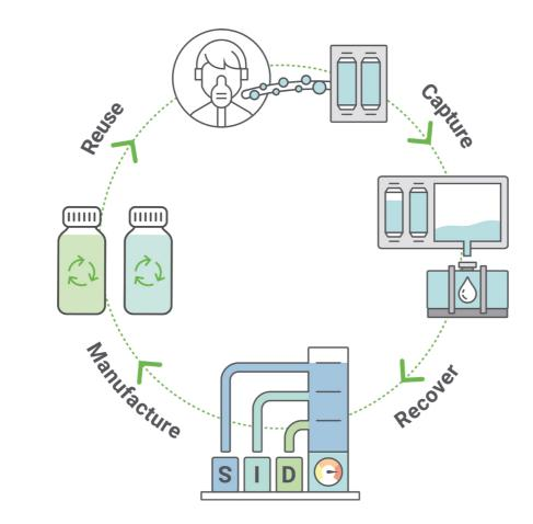
capture technology, the recovery process, and the remanufacture processes. The solution is most sustainable when deployed at large scale. Bringing the capture, recovery, and remanufacture of volatile anaesthetics scaled for global reach in a highly regulated industry is also innovative. The project is important as the emissions from the use and disposal of volatile anaesthetics contribute four million tonnes of carbon dioxide equivalents each year.
