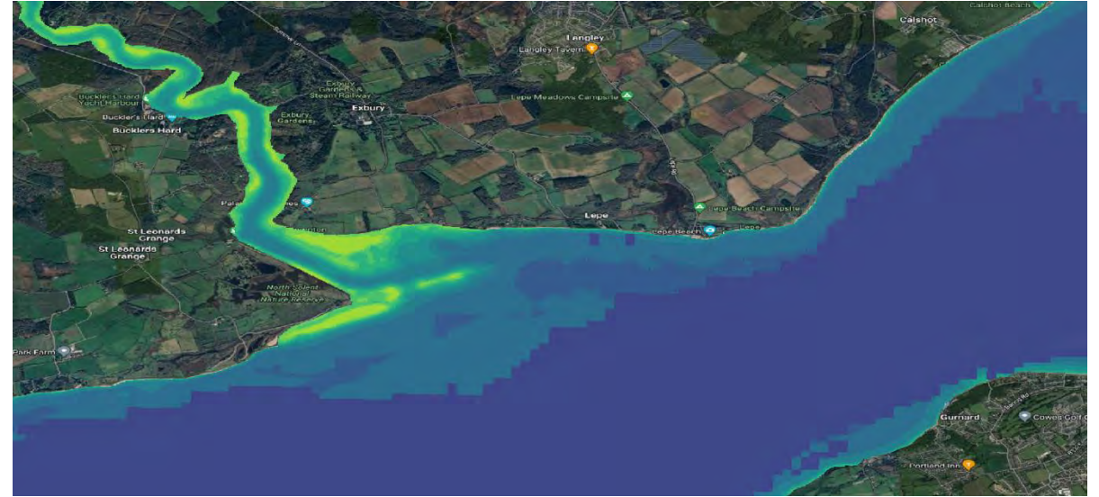
The Solent: Precision water depth measurements.
