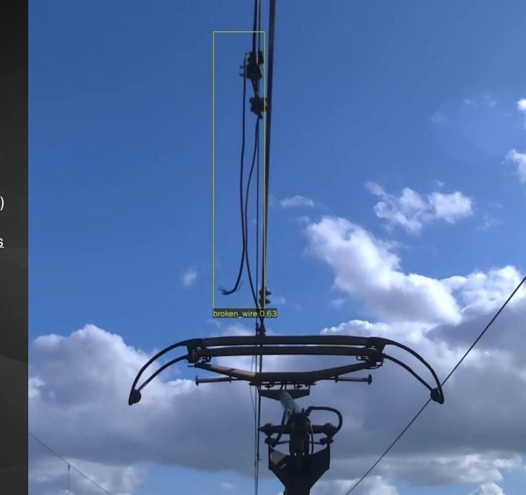
1. Al Dropper Wire Fault Detection
