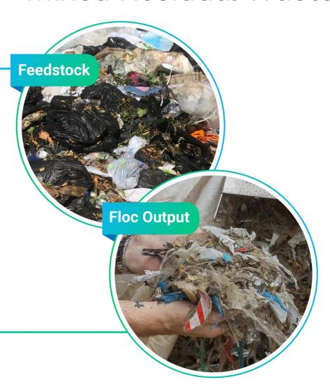
Waste is treated in the machine for approx 3 days, this is the typical results for the floc
