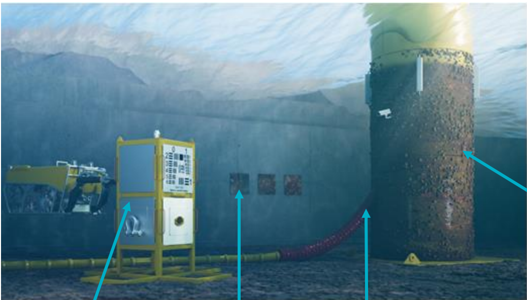
Visual and manipulation test piece including visual panels, handles etc
