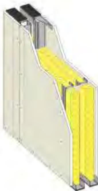
Conventional internal partition wall 45dB acoustic reduction
